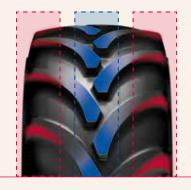
lug in the center in driving direction for comfort and wear resistance.
